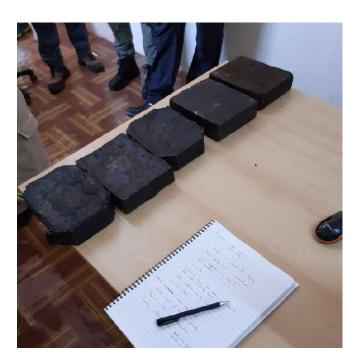
Photo 2. Experimental bricks manufactured using recycled plastic
