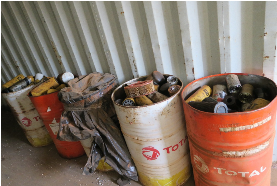
Photo 7. Waste solvents in a sealed container – strong solvent vapours
