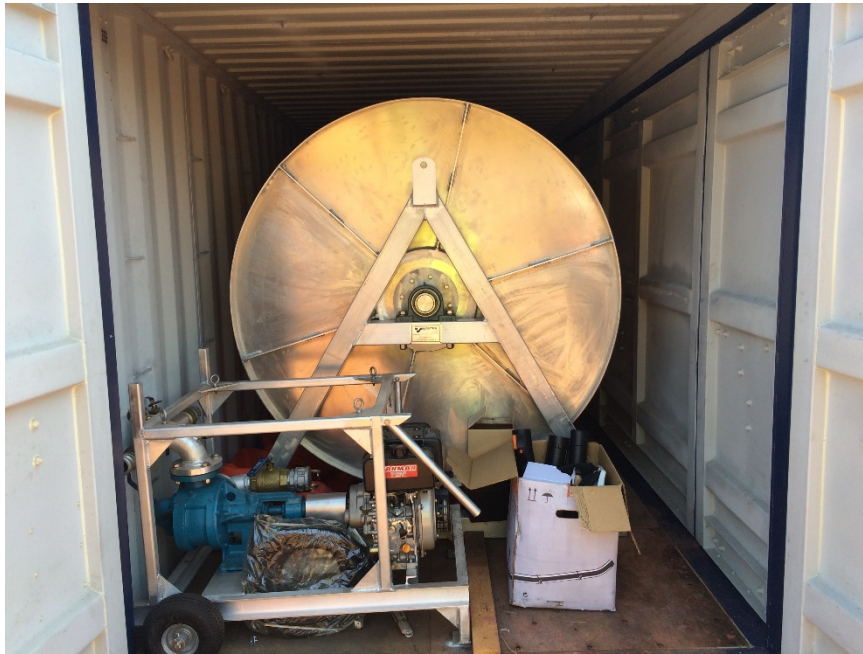
Photo 23. Heavy duty oil boom – suitable for offshore
