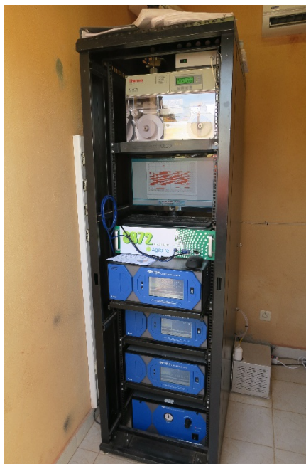
Photo 12. Continuous air quality monitoring equipment
