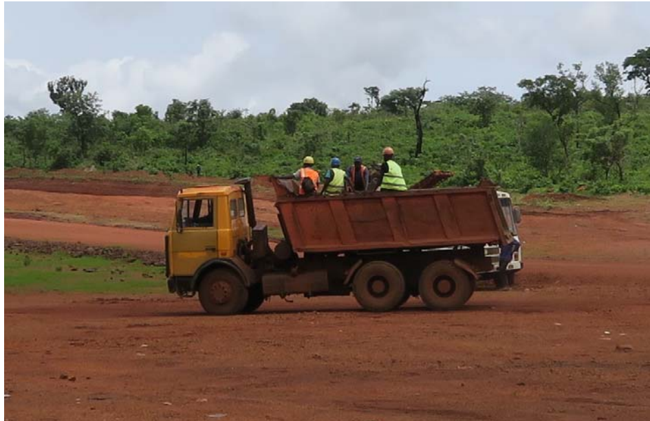
Photo 15. COBAD Road - poor H&S practices are common place
