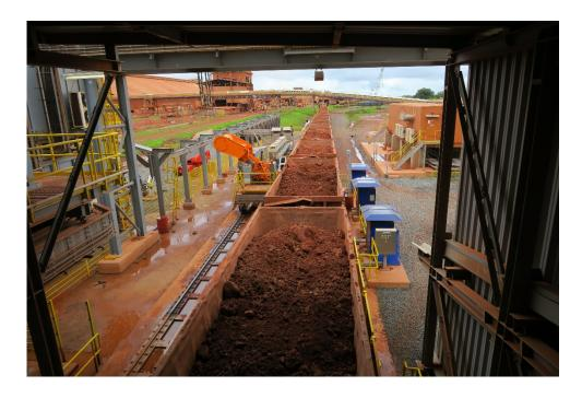
**Photo 11.** Rail wagon entering new tippler
