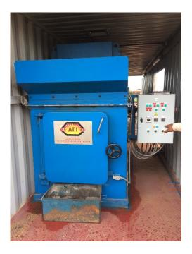
**Photo 3.** Newly installed incinerator at Tora Bora waste facility
