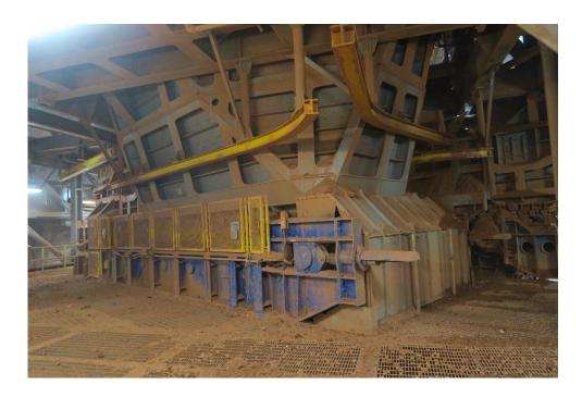
**Photo 13.** Crusher in base of pit
