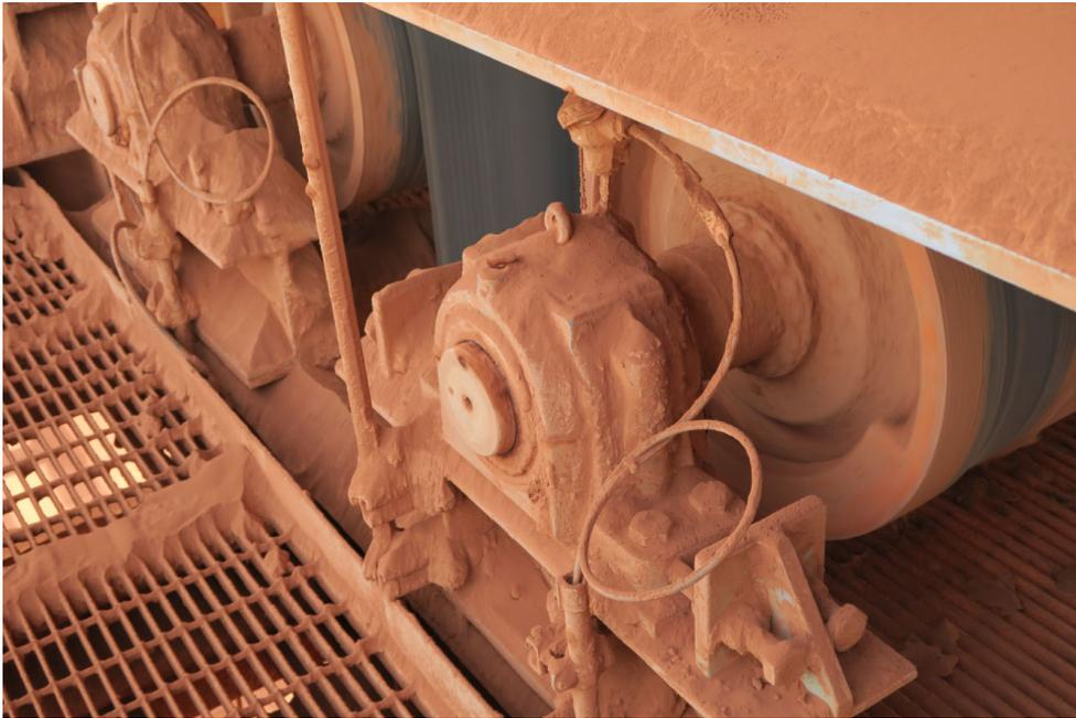
**Photo 27.** Rotating machinery at ankle level adjacent to walkway – consider safety screen
