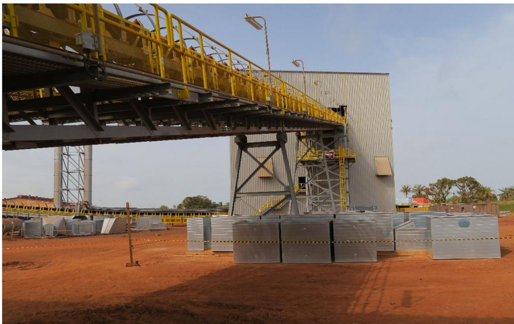
**Photo 4.** Conveyor and secondary sizer
