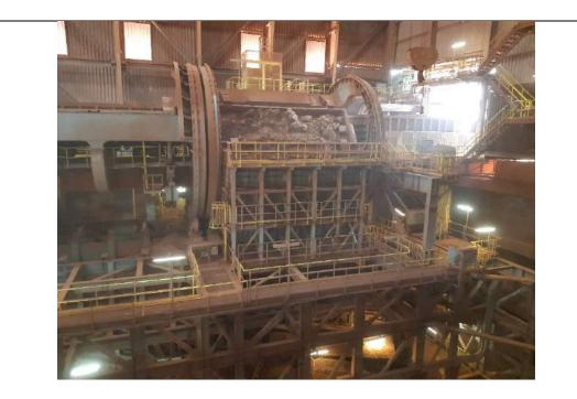
Photo 21. Tippler – rotating wagon emptying laterite into primary crusher
