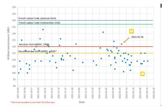
Figure 7-5. Overblast pressure measured in villages during blasting events
