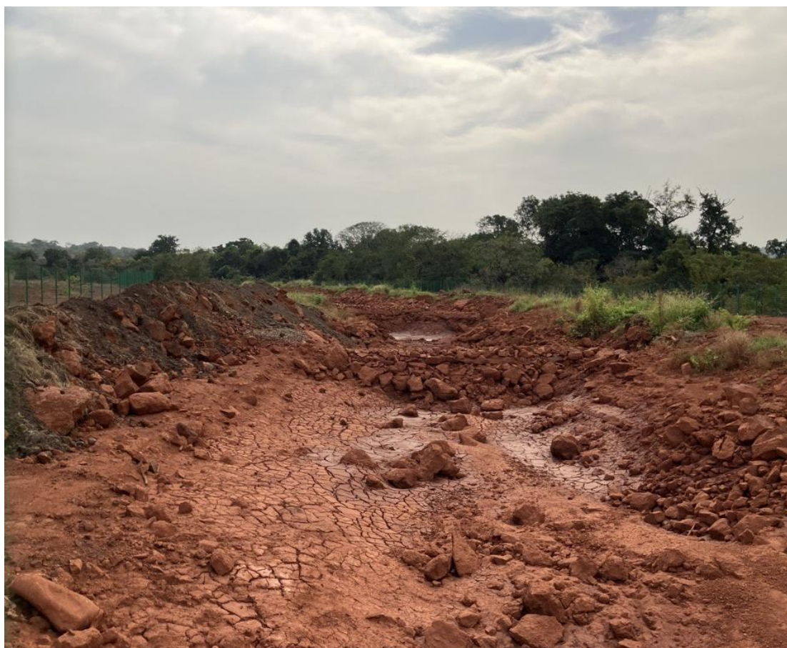
Figure 8-4 Sedimentation basins on the Kagnaka plateau (zone which will be mined in the future)
