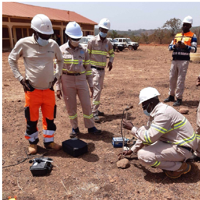
Photo 8. Noise monitoring during blasting event, Fassaly Foutabhé
