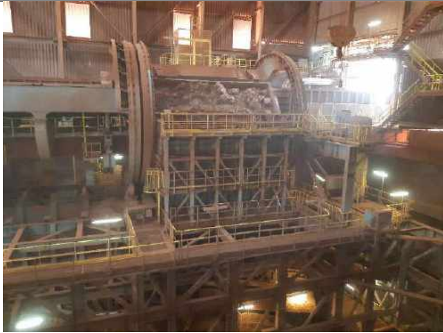
Photo 21. Tippler – rotating wagon emptying laterite into primary crusher
