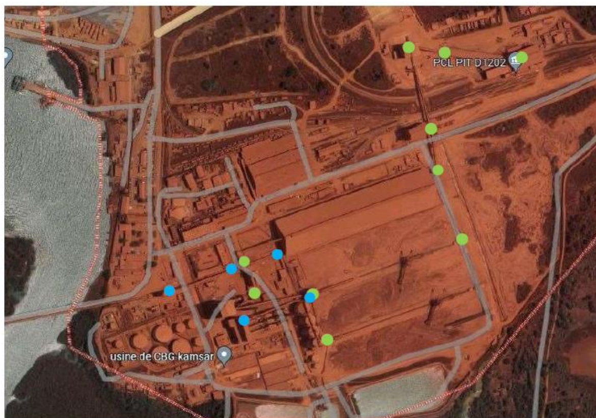
Figure 8.5: Location of existing (in green) and new (installed in January 2024, in blue) dust suppressing points at Kamsar Plant
