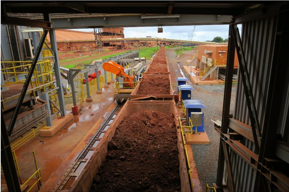
**Photo 11.** Rail wagon entering new tippler
