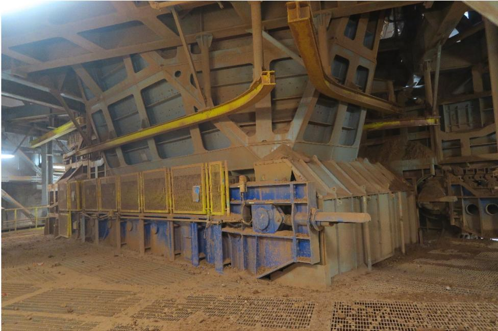
**Photo 13.** Crusher in base of pit
