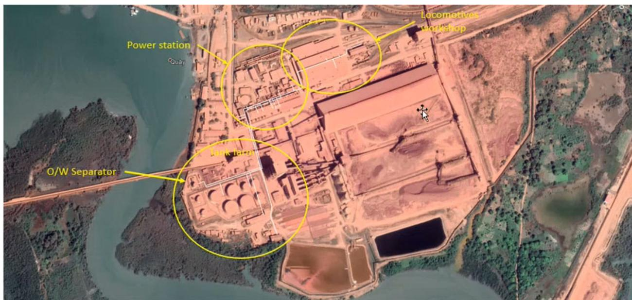
**Figure 7-4. Aerial image showing location of oil generating facilities and effluent system (white lines)**
