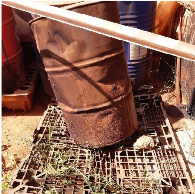
**Photo 7.** Damaged secondary containment resulting in unstable storage of corroding drums (site adjacent to the old oil waster separator)
