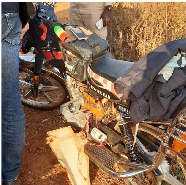
**Photo 20.** Use of motorcycle battery to charge mobile phone
