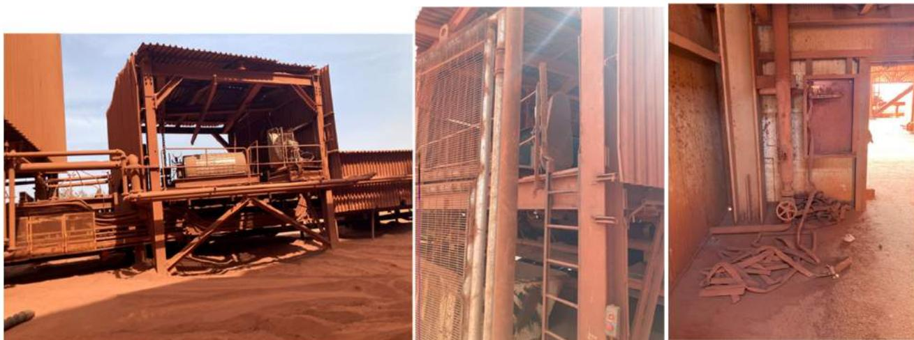
**Figure 6-1 “Déferailleur”(Carter Missing or Defective) and Fire Hoses Broken on the Floor**
