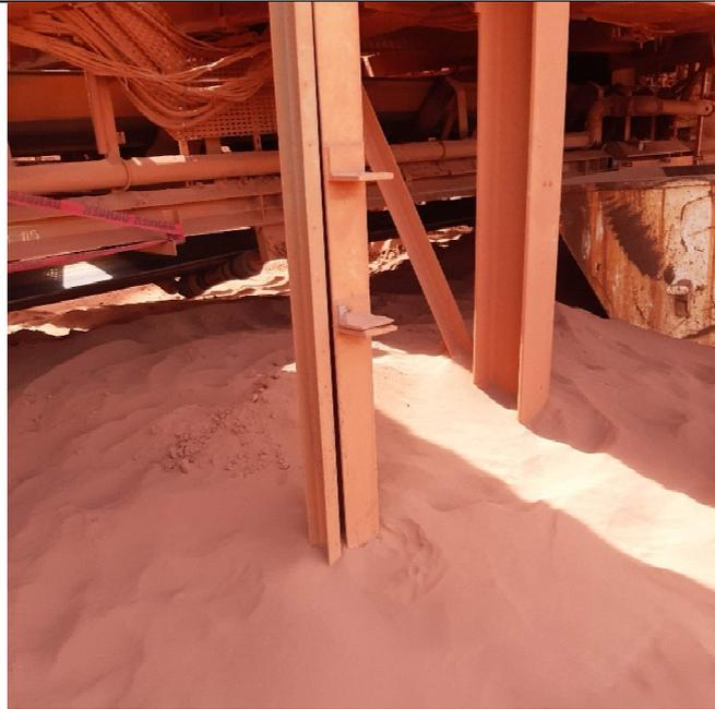
**Photo 25.** Accumulated dust beneath conveyors/moving machinery at Kamsar
